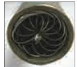
Finned Tubing Cross Section
